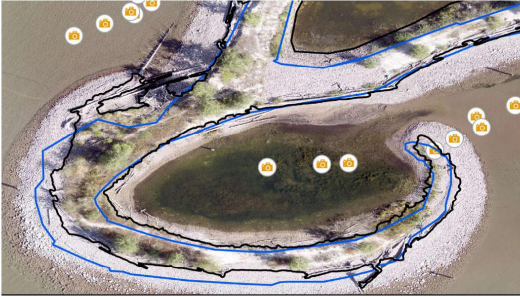
Figure 53. This aerial photograph of the spit embayment shows the extensive regrowth of aquatic plants within the spit embayment. It also shows the areas of erosion and deposition since 2016 on the outer lakeward shoreline (difference between blue 2016 and black 2023 shorelines). The gravel beaches in this area are exposed to the highest levels wave action for the entire WPA constructed shoreline.
