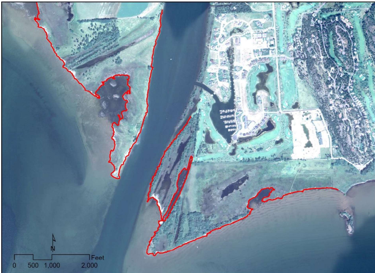
Figure 1. This is a 2005 MT Department of Natural Resources airborne NAIP image of the north shore showing the USFWS Waterfowl Production (WPA) prior to the construction of erosion control structures that began in 2007 along what is now the MTFWP Osprey Landing property (see figure 4). The red line is the shoreline at that time and represents the limit of shoreline loss prior to construction of the both shore-attached, and offshore erosion control gravel beaches and gravel, large wood erosion control structures built to stop erosion to the WPA riverbanks. This line serves as a metric in the analysis of structure success in the 2016 and 2017 final reports to the EKI and are included in this final report. Success is defined then as maintaining this shoreline position. Construction of erosion control structures started in 2007 on the eastern edge of the WPA extending to the river mouth in 2009. Construction of erosion control structures was completed for both sides of the river mouth by 2012.
