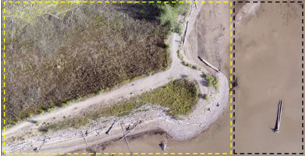
Figure 35. This aerial drone image taken in August 2023 photo shows a revegetated spit embayment and wetland complex behind it. The area in the yellow box looked just like the barren lakebed within the black box prior to construction of the gravel dikes. This photo area is shown as a yellow box in figure 36.
