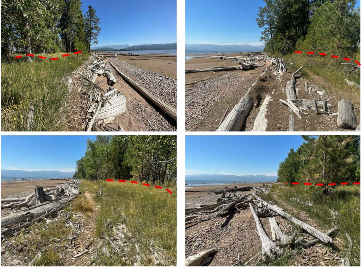
Figure 50. These four photographs show the current 2023 condition of the shoreline on the lakeward side of the eastern WPA. This section of shoreline has been accreting since construction of the shore attached gravel beach in 2008. The deposition of windblown sand and logs followed by riparian succession of plants results in the creation of new, dynamic shoreline habitat. The red dotted lines show the approximate position of the 2005 shoreline.
