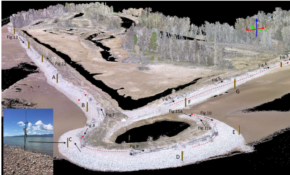
Figure 2. This graphic, from the 2017 final report is a color enhanced, 3D oblique aerial view of the offshore beach and spit just east of the river mouth. This DEM was derived from drone-based LiDAR data and imagery collected May 5 th , 2017. The water appears black and the exposed lakebed tan to light brown. The location of pilings driven into the lakebed are shown with labels near those where cross-sectional profiles are compared between May and Oct LiDAR data collections. Location of photographs are shown by corresponding Fig. # with black arrows showing the view orientation. The red dotted lines with arrows show the direction of gravel transport. The photo inset shows the weather station located at piling C.
